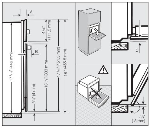
A <sup>7</sup>/<sub>8</sub>" (Appliances with glass front: 22 mm / Appliances with metal front: 23 mm)
